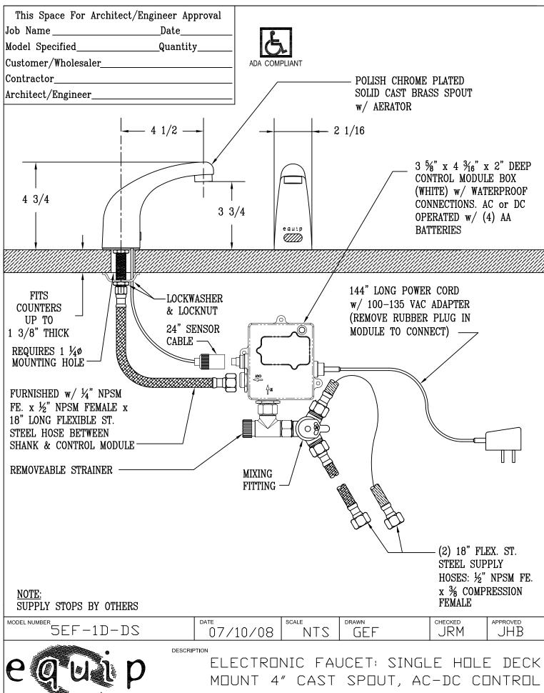
equip Foodservice Accessories P.O. BOX 1088, 2 SADDLEBACK COVE TRAVELERS REST, SOUTH CAROLINA 29690 PHONE: 800.891.4808 FAX: 800.868.0084 MODULE, TEMPERATURE CONTROL, MIXING VALVE, AND 18" HOT & COLD FLEXIBLE SUPPLY HOSES
