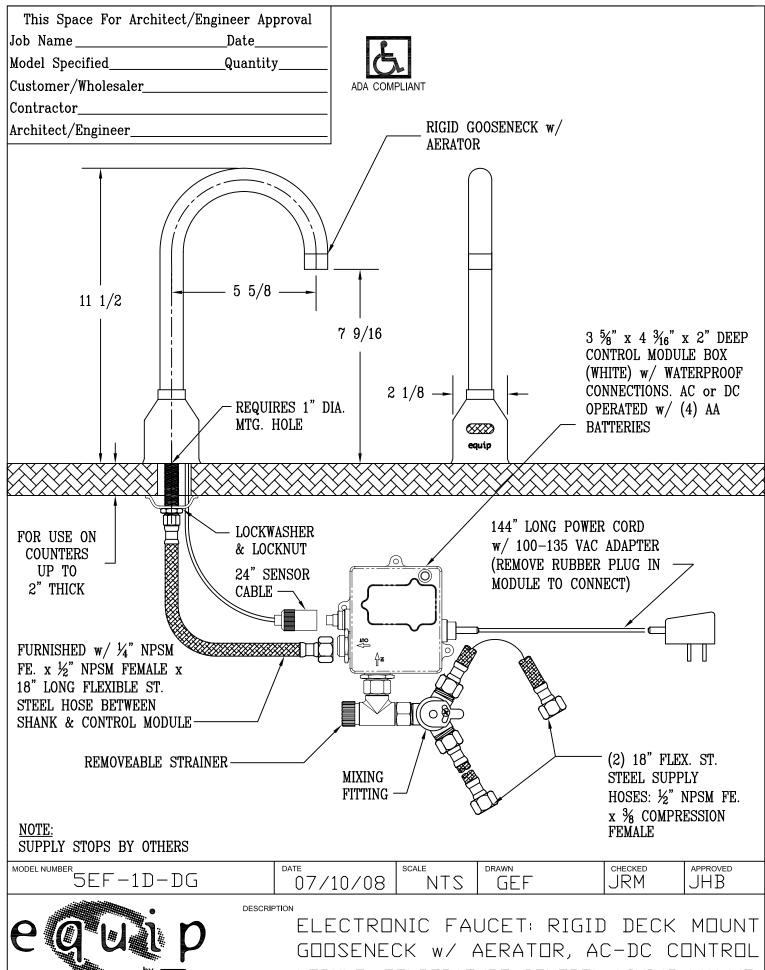
equip Foodservice Accessories P.O. BOX 1088, 2 SADDLEBACK COVE TRAVELERS REST, SOUTH CAROLINA 29690 PHONE: 800.891.4808 FAX: 800.868.0084 MODULE, TEMPERATURE CONTROL MIXING VALVE, & 18" LONG HOT & COLD SUPPLY STOP FLEX, CONNECTORS
